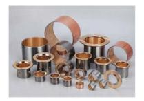
Steel shell backed with a lead bronze lining bearing material for oil lubricated applications. This material has high load capacity and good fatigue properties. It is widely used in automotive applications such as compressors, steering gear, power steering, pedal bearings, king-pin bushes, tailgate pivots, mechanical handling and lifting equipment, hydraulic motors, agricultural machinery etc.
